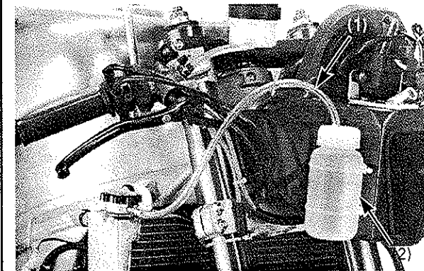
(1) OVERFLOW TUBE (2) CATCH TANK
